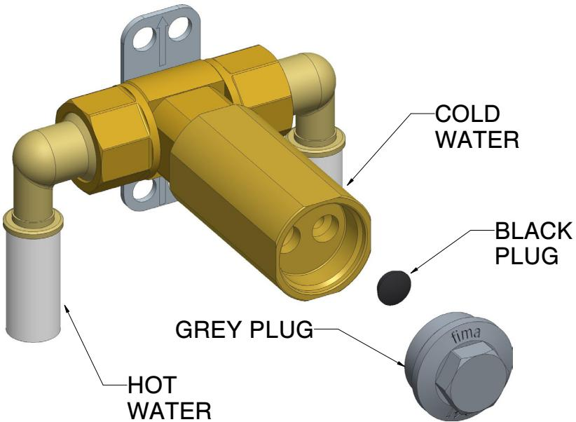
**STEP #2 :** Once the hot and cold inlets have been connected you need to flush the pipes to make them perfectly clean. To do that, just remove the grey plug and open both hot and cold bathroom principal valves for a short time. Then close them and remount the grey plug.
