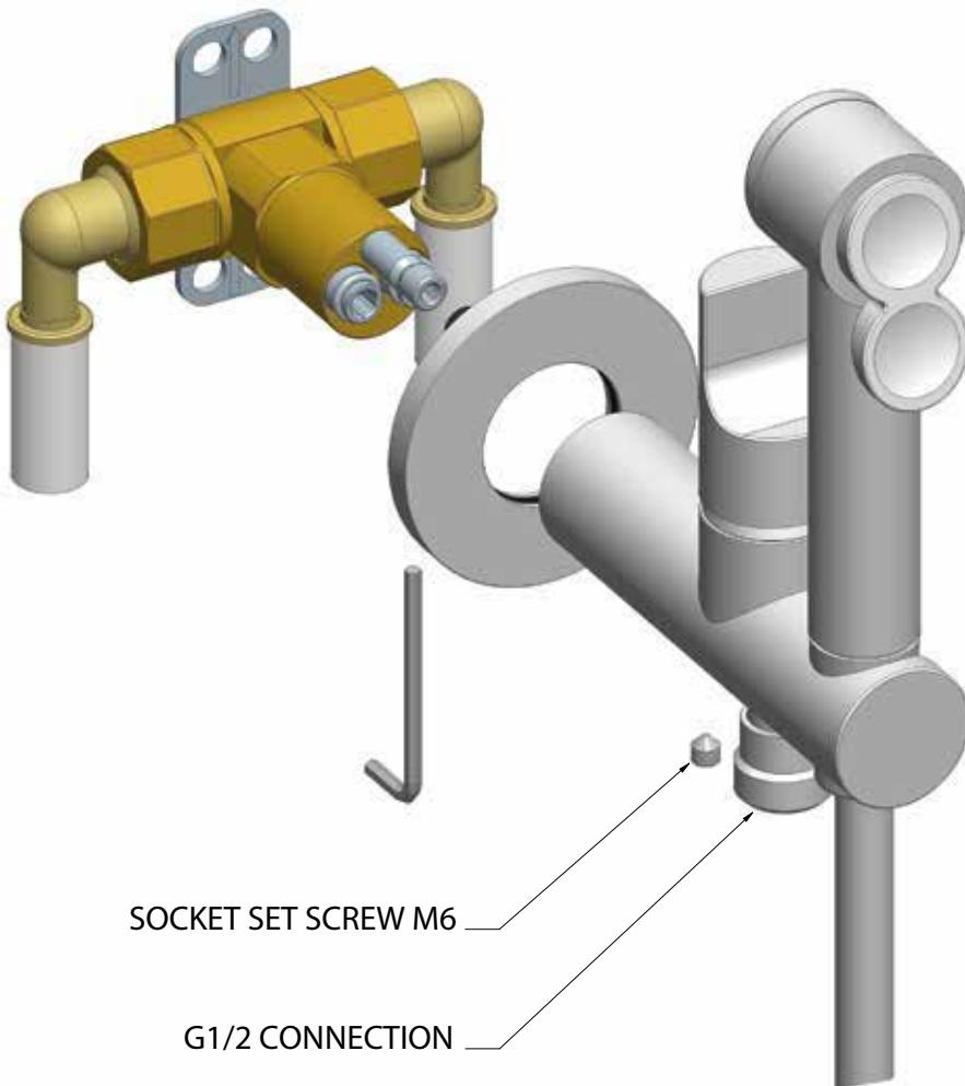
STEP #5 : After removing the cover, mount the rosette over the external body and insert the complete external part in the built-in part, fixing it with the M6 socket set screw included. Then connect the flexible hose to the handshower and to the G1/2 threaded connection. See figure above.
