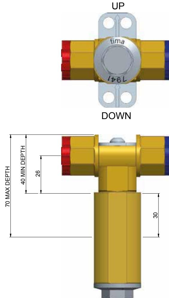
STEP #1 :Install the built-in body respecting the indication of the label about MIN and MAX depth of installation. Pay attention to the right orientation of the body itself (small arrows on the inox plate pointing up) and use a water level to adjust the horizontal positioning. See figure above.
